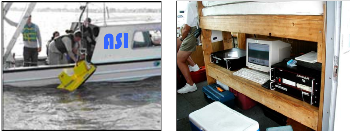
Figure 15. Edgetech X-STAR sonar system. SB-216S towfish is shown on the left and topside amplifier, computer monitor, and digital recording system is shown on the right.
